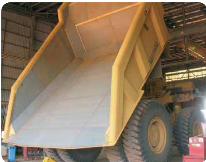
Matrox coils: Ideal for lining on road dump-truck beds.
