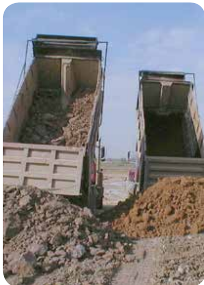
Comparison between Matrox and steel. The material adheres to large areas of the unlined steel surface. The area lined with Matrox is almost completely free.
