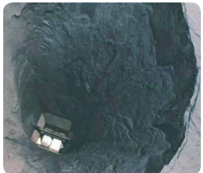
Funnel Flow: The flowing material (dark grey) is forming a funnel, while the rest (grey) is sticking to the walls of the bin.
